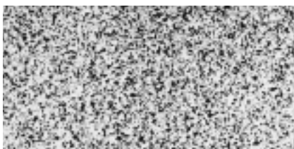
Querschliff Ag/C Cross section Ag/C Coupe transversale Ag/C
